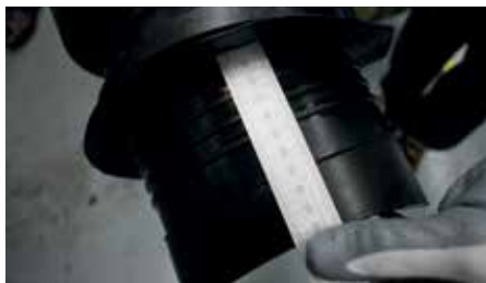
Adjust the screw collar according to the wall thickness.
