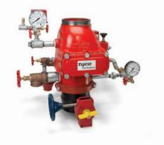
The Model DPV-1 Dry Pipe Valve is a differential valve that can be used to automatically control the flow of water into a dry pipe fire protection sprinkler system upon operation of one or more automatic sprinklers.
