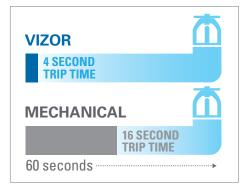
Quick, consistent valve trip provides a much wider margin to meet the 60-second code requirement for water discharge at the most distant sprinkler head. LOWER LABOR COSTS
