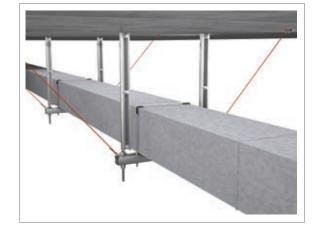
International seismic standards accept the use of both cable and rigid bracing. Cable bracing has the advantages of being versatile, lightweight and easily transportable.
