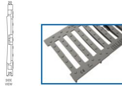
SLOTTED GRATING 20 mm DIMENSIONS L x I x h DRAINAGE SURFACE OPENINGS F1 x F2 CODE MATERIAL WEIGHT PRICE FIXING SYSTEM dm² € mm kg mm tie-tod no fixing GJS 500/7<sup>6</sup> ductile iron water based paint coated up to Class C250 as per Standard EN 1433 502124 180,0 x 20,0 498 x 248 x 20 7,00 4.32
