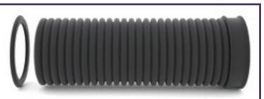
The **pipe** is a high density co- extruded twin wall pipe, smooth internally and externally corrugated with stiffness class SN8  $kN/m^2$  (on request it is possible the class SN 16  $kN/m^2$ ).
