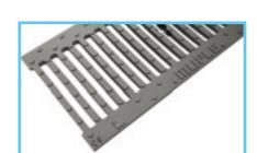
SLOTTED GRATING 13 mm DIMENSIONS L x I x h DRAINAGE SURFACE OPENINGS F1 X F2 CODE PRICE MATERIAL WEIGHT FIXING SYSTEM € mm dm² mm no fixing kg tie-tod GJS 500/7<sup>6</sup> ductile iron water based paint coated up to Class C250 as per Standard EN 1433 500155 180,0 x 13,0 498 x 254 x 7 7,20 4,68
