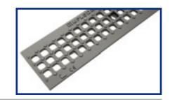
DIMENSIONS L x I x h OPENINGS F1 X F2 WEIGHT CODE PRICE MATERIAL FIXING SYSTEM no fixing € mm kg tie-tod mm GJS 500/7<sup>6</sup> ductile iron water based paint coated up to Class C250 as 506101 498 x 135 x 7 3,30 2,15 21,0 x 17,0 per Standard EN 1433
