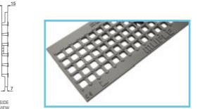
DIMENSIONS L x I x h DRAINAGE SURFACE CODE PRICE MATERIAL WEIGHT OPENINGS F1 x F2 FIXING SYSTEM € mm dm² tie-tod no fixing kg mm up to Class C250 as per Standard EN 1433 GJS 500/7<sup>6</sup> ductile iron water based paint coated 500149 498 x 204 x 7 4,70 3,58 21,5 x 17,5
