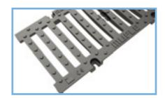
SLOTTED GRATING 20 mm DIMENSIONS L x l x h OPENINGS F1 x F2 DRAINAGE SURFACE CODE PRICE MATERIAL WEIGHT FIXING SYSTEM screw € mm kg  $dm^2$ mm GJS 500/76 503115 ductile ironwater based 498 x 248 x 25 8,20 4,32 182,0 x 20,0 paint coated
