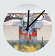
After 8 minutes, approx. 625 °C: the pipe is melted; the swelling mass fills the entire barehole
