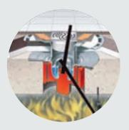
After 25 minutes, approx. 800 °C: borehole and connection are completely sealed. The water trap remains largely in tact.
