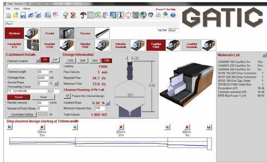
Gatic Slotdrains designed in DrawNet using graphical user interface in 3D worldview
