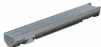
FILCOTEN SELF Domestic Channel NW100 with Galvanised Steel Heelsafe Narrow Grating (A15kN)
