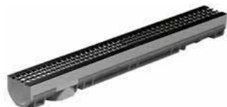
FILCOTEN SELF Domestic Channel NW100 with Ductile Iron Grating with Snap-On locking (B125kN)
