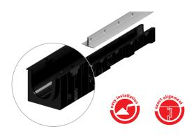
BrickSlot H80 "T" section is designed for **EASY 100** channel made of HD-PE with no rails. The absence of the rail ensures that the grating completely covers the channel. BrickSlot H80 "T" section can be installed on Easy 100 in all its internal heights: 55, 80, 100 and 160mm.
