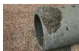
pipes with irregular surface
