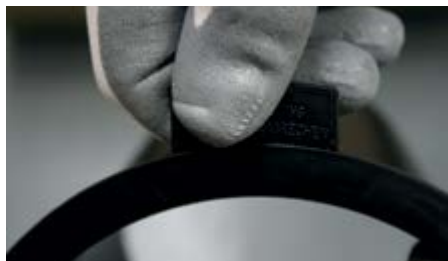
Remove the transport lock from the clamping sleeve. Water the clamping sleeve and the element.
